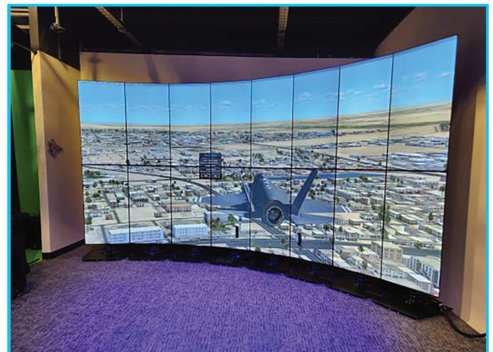
Hydra Stands with double 55" monitors in a curved 2X8 Video Wall
